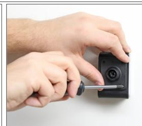
Place the base plate over the matching holes in your mounting bracket (demo ProClip mount shown in picture) Attach the base plate by using the self-tapping screws. Note: The machine screws with nuts are for mounts made of metal with large holes.
